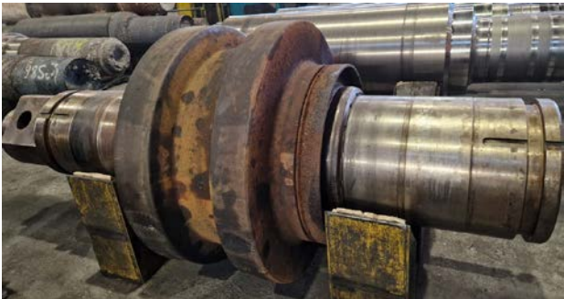
↑ → Edger rollers in hot strip mills are susceptible to wear
