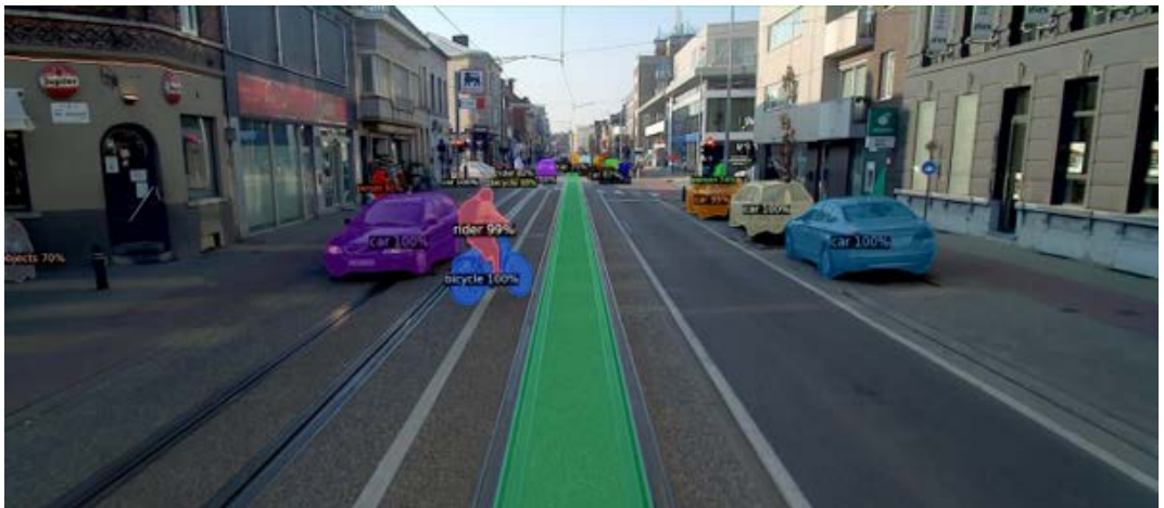
↑ Real-time object detection and track segmentation: OTIV's vision system at work in an urban tram environment.
