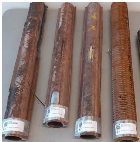
↑ Sampled boiler tubes (left); section cut of a clogged boiler tube (right)
