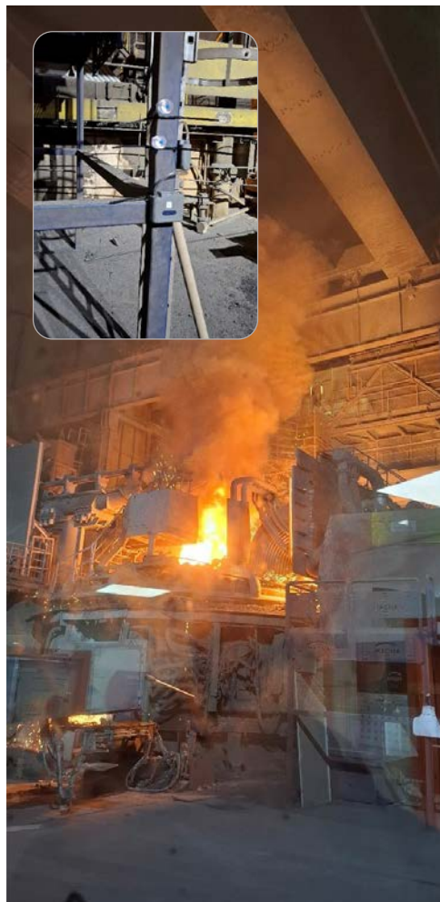
↑ EAF production and detail of the dust sampling devices (pumps and filters)
