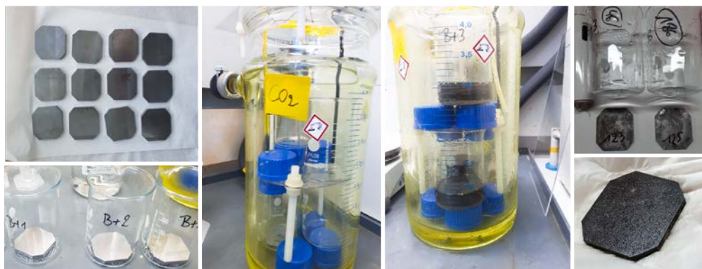
↑ Severe corrosion of corrosion coupons exposed to the typical acid composition that can be formed in a CO 2 high pressure operating pipeline
