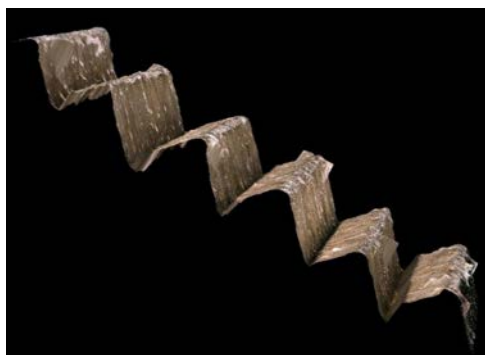
↑ 3D surface scan (left) and false-colour topographic map (right) revealing the quality of a stack of coated laminations.
