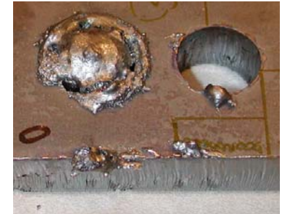
Poor laser cut
